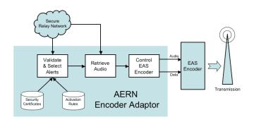
The AERN Encoder Adaptor connects to the encoder in the same way as an ordinary encoder control unit. It monitors the relay network for incoming AERN (CAP) messages, authenticates and selects received alerts by location and category, retrieves the recorded audio, and then extracts EAS header data from the CAP message and triggers the EAS encoder. Transmission can be automatic or it can require manual operator approval, as dictated by station/system policy.
