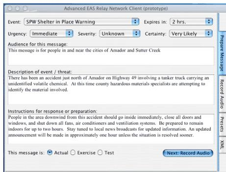
The main message entry screen prompts the originator to compose the elements of the EAS message. Additional parameters used in the CAP message format, such as the urgency, severity and certainty values, can be adjusted as necessary, although in most EAS applications the supplied default values will be correct.
