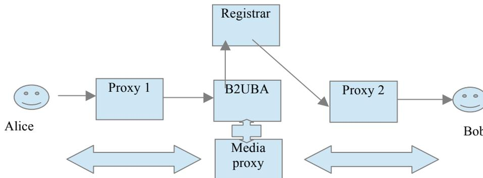
In the diagram above, the subsystem that is aware of the nature of Bob is the registrar. The subsystem that is able to execute the core of the call procedure is the B2BUA. The call procedure needs to be augmented as follow:
